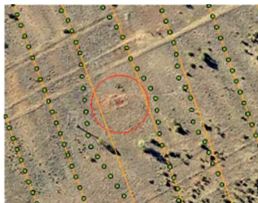
Figure 13. Image that shows a cultural heritage exclusion area (in red) through which the original, 24 m spaced, lines (in orange) clearly cut. The green circles show the lines after the application of the planning algorithm. They avoid both the exclusion area and the adjacent trees.
