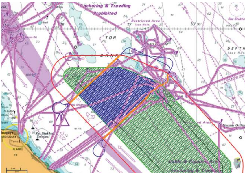
Figure 5 OBN design around obstructed area and shipping lanes, showing 200 x 200m receivers, with H pattern roll. Shots for the current patch are shown in orange, with active receivers in blue.
