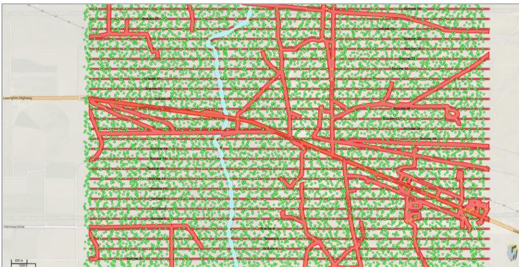
Finally, a roll pattern was created such that the project could be acquired with 2 swaths using 96,000 receiver nodes. The resulting high resolution, long offset, full azimuth design delivers trace densities up to 70M traces per square kilometer. Note that this technique can also be used for seabed node projects.
